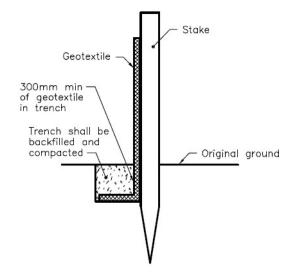
**GEOTEXTILE: 36" Black Woven Geotextile**
