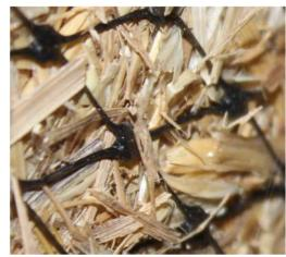
DNSC is manufactured using 70% agricultural grade wheat straw and 30% biodegradable coir fiber that is bound and sewn between 2 layers of polypropylene netting. DNSC is excellent at holding seeds and soil in place while vegetation is developed. As it biodegrades over time it releases beneficial nutrients to the soil to help further increase vegetative development. It also absorbs water while still maintaining its structural integrity.
