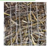
The information below summarizes the product's typical physical properties at the time of manufacturing. Manufactured using 70% agricultural grade wheat straw and 30% biodegradable coir fiber that is bound and sewn between 2 layers of natural organic netting.
